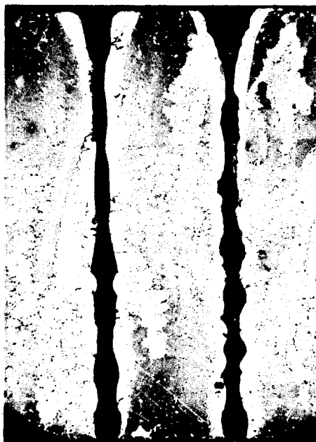
Less than a third of the 100-diameters length of the holes is shown. Holes are bell-mouthed and irregular at entrance end (top of picture) and are irregular in cross section. (Compare with holes produced by laser beam machining, shown on page 256.) Cracks extend to a depth about equal to the hole diameter.
