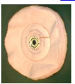
Canton flannel is very soft, and this wheel is loosely stitched, so the layers of cloth flare out to give a wide angle ultra smooth polishing surface.
