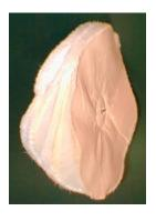
The main purpose of a loose cotton wheel is to polish and cut in a similar manner to the Spiral sewn wheel, except that this wheel, not being tightly stitched together, will 'mush' or collapse, allowing the cotton to get into awkward places more easily. If you have an object with fine details and awkward crevices, then this is the wheel to use.
