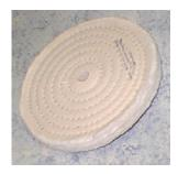
Spiral sewn wheels are the workhorse of most buffing and polishing jobs. Because the ply's of cotton cloth are sewn together spirally, the wheel becomes much harder and more pressure can be exerted on it. This is especially useful when 'cutting' the metal.
