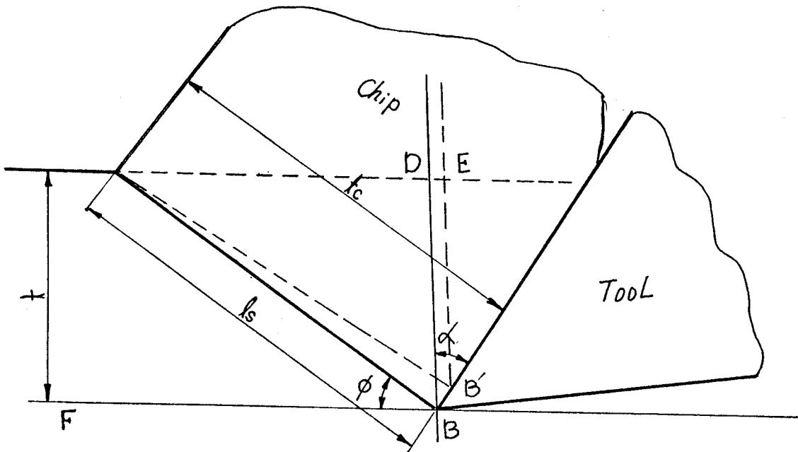
$$T_s = (F_c \cos \alpha - F_t \sin \alpha) \cdot \sin \phi / t_{bw} \quad \dots \textcircled{1}$$
