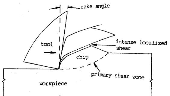
Fig.3 Model of a shear-localized chip formation process.
